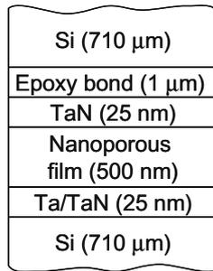
Fig. 2. Schematic illustration of a sandwiched multilayer thin-film stack.
